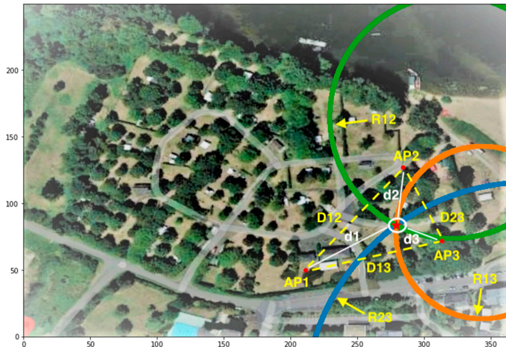
Figure 5. Circles of Apollonius (green, blue, and orange) for AP1, AP2, and AP3, separated by distances D12, D13, and D23. A client within the white circle sits at distances d_1 , d_2 , d_3 from the three APs. The radii of the circles are R_{12} , R_{13} , and R_{23} . The solution for the client location determined from the RSS values at the three APs is indicated by the red star at the intersection of the circles.
